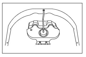
3. Remove the wheel stow rod from the upper left side of the floor compartment.
